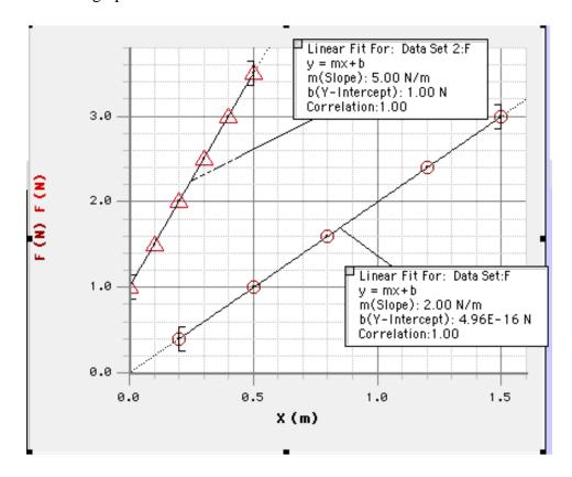
a. Write the equation that describes the relationship between the force and the stretch of **spring 2**.
